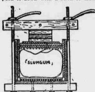
CROSS SECTION OF WAX-PRESS fit on the bottom and in the corners. Fold up the mouth of the sack and the sheet over it. Put the follower on, with the blocks on top. Swing the cross-bar over and push the screw up through the hole in it. Put on the handle and turn both handles down, one at a time.
