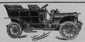
Five passenger Touring Car, 4 cylinder 43/4x43/4, 32 Horse Power. Transmission—Selective Type, three speeds, forward and reverse. 34 inch wheels, 4 inch pneumatic tires, 112 inch wheel base.
