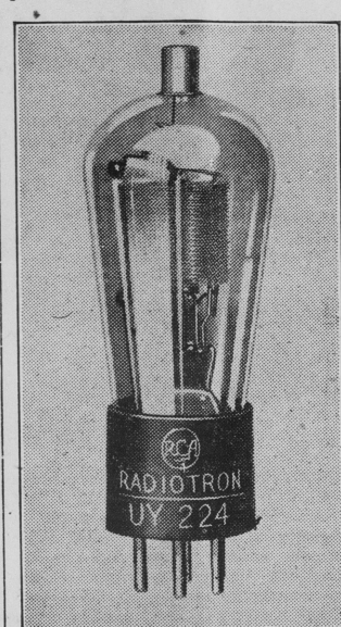
A four electrode, screen grid tube, with new features.
