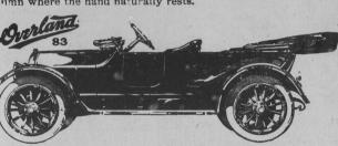
35 horsepower motor. High tension magneto ignition. Electric starting and lighting. Left-hand drive, center control.
