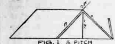
Fig. 1 is what is known as one-half pitch, one-half the height of width, and if a hip roof is wanted the rafter would be 20 feet and six inches long.
