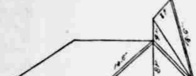
Fig. 2 is one-third pitch, one-third the width.
