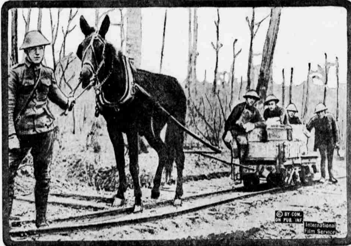
Transporting food on a narrow-gauge road, car hauled by mule, to the trenches under cover of dense woods.
