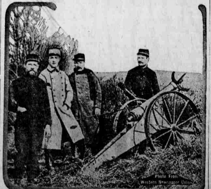
This French gun throws an anchorlike projectile into the barbed wire defenses of the enemy. The missile is attached to a cable and is hauled back to be fired again and again.
