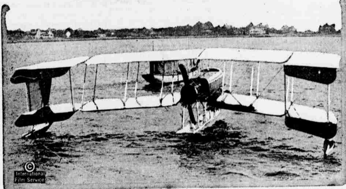
This wireless-control airplane has just been built by the Burgess-Curtiss company for John Hays Hammond, Jr., and will be given a series of tests for the United States government. According to the inventor's plans, the operator can "pick up" a torpedo and, by means of the wireless-control outfit placed just back of his seat, can direct it against the object of attack.
