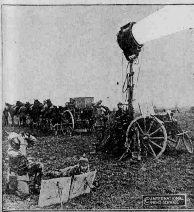
One of the German field searchlights which are so useful in guarding against attacks from the air. The officer in the left foreground is observing an enemy aeroplane, his instructions being sent by the telegrapher at his side to the nearest artillery position.
