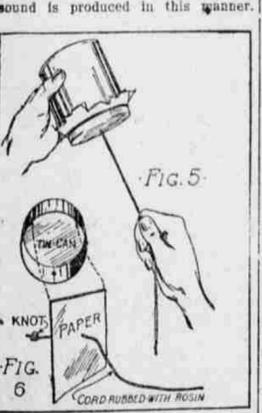
Figure 5 shows the idea adapted to a toy that is quickly put together. Get an empty tin can, a piece of heavy wrapping paper, a piece of stout twine, and a piece of resin.
