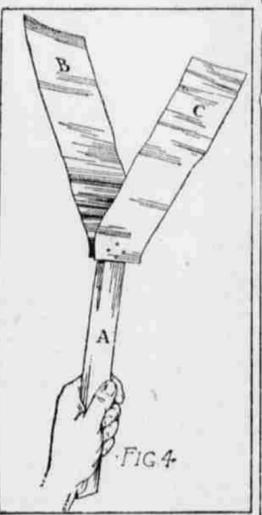
By holding the handle in the position shown in Fig. 4, and shaking from side to side, the tin wings will flap back and forth and make a splendid crackling, crashing noise.
