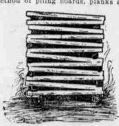
small dimension lumber. Inch strips for edgings are placed near each end, and in the middle of the pile. top course of boards is put on in the form of a roof to shed the water Very useful methods of piling ties, posts and other timber are shown in
