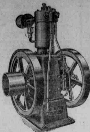
The Gasoline Engine is one of the most useful things a farmer can own. With one of these useful machines he can saw wood, grind feed, shell corn, pump water, and many other things.
