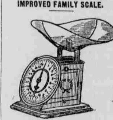
Improved Family Scale. The illustration shows an improved family scale of the dial type, the particu- lar feature of which is the slanting position of the dial, thereby enabling the indications of the pointer to be read with greater facility. The ordinary vertical dial requires the user to bend over in order to distinguish with any degree of accuracy its indications. In other particulars the scale conforms to the conventional design of this type.— Philadelphia Record.
