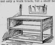
low it for keeping tools. The cover of the box can be hinged to the front for the purpose of keeping the tools more secure. There is not a farm in the country that can afford to be without at least a small bench on which to make repairs and to construct the small articles needed in carrying on farm operations.-New York Tribune Farmer.
