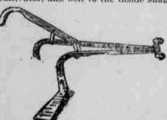
on each side a horizontal kulfe eighteen inches long and sloping back slightly. The knife is shown in position in the illustration (one handle removed) and is made from one of the knives from an old stalk cutter. This attachment is used by the Kansas Experiment Station quite successfully. Any blacksmith can make it.-American Agriculturist.
