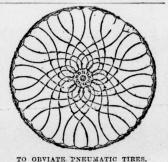
degree the use of pneumatic tires. His latest design is shown in the accompanying illustration. The wheel is constructed of Sheffield steel, with an ordinary cushion tire and twin-spring spokes, "having perfect lateral rigid-ity without vibration." The idea evi-dently is to take up the vibration in the wheel itself, instead of in the tire, with the thought of dispensing with pneumatic tires, with their liability to puncture.
