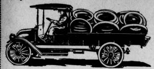
International Motor Truck, Model "F," 2000 lbs. capacity, four cylinders cast en bloc, left hand drive, center control, shaft drive.
