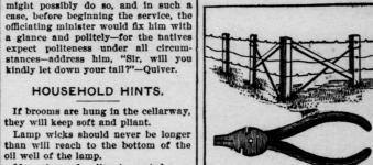
WIRE FENCE TIGHTENED. wire will "sing" and be tight. It is a good way to make the wires all tight alike, and I think it is a good plan to kink the wires in a new fence, espe-cially smooth wires, for they will not be so apt to break from contracting by cold. If any person who reads this article has loose wire fence, just get you pliers and try it. The cut illustrates the method of kinking.
