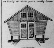
ed. The cribs may be made from six to eight feet wide and of any desired length. For 4,000 bushels of corn in the ear the building should be 40 feet long with cribs 8 feet wide and 12 feet high. In building this one should use 6 by 8 timber for sills and 2 by 8 joist.
