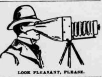
nary square focusing cloth. It is made slightly larger at one end than the ground glass, and an elastic band is sewed in that end. This fits on the camera, and need not be removed during the taking of the picture. An elas lic band at the other end holds the cloth against the operator's face. Another advantage is that it is not necessary to use one hand to hold the cloth at the bottom to exclude the light.
