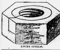
keep the first one from unscrewing. ed a dime for old acquaintance sake, the second nut being called the jamnut, or lock-nut. The clastic nut, however, locks itself
