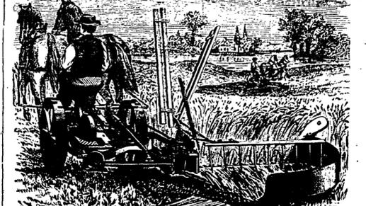
DODGE'S PATENT REAPER AND MOWER, AND SELF-RAKING HARVESTER. OHIO AND BUCKEYE COMBINED. WITH DOUBLE DRIVING WHEELS, & SELF-RAKING CUTTING APPARATUS.
