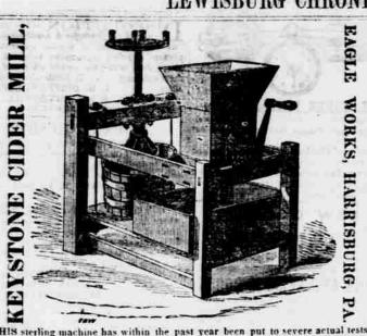
THIS sterling machine has within the past year been put to severe actual tests, and been very much improved by the addition of a 22 inch fly wheel, new gearing, joint bolts, and other minor improvements, and is now offered to the public with the certainty that it is made in the very best manner, and that it will grind and press easier and faster than any other Mill in the market. Dealers and others supplied on liberal terms.
