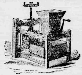
N the present groungement of this highly approved and valuable WILL the labor is divided by arranging a cutting Cylinder to break the applies, and then deliver them to the lower cylinder to be reduced to pomace. By this arrangement the work is performed faster and with much less
