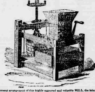
N the present arrangement of this highly approved and valuable MII.L, the labor is divided by arranging a cutting Cylinder to break the apples, and then deliver them to the lower cylinder to be reduced to pomace. By this arrangement the work is performed faster and with much less
