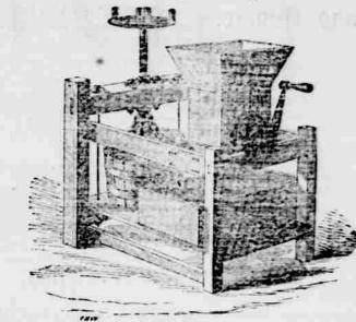
In the present arrangement of this highly approved and valuable MILL, the labor is divided by arranging a cutting Cylinder to break the applies, and then deliver them to the lower cylinders to be reduced to pomace. By this arrangement the work is performed faster and with much less
