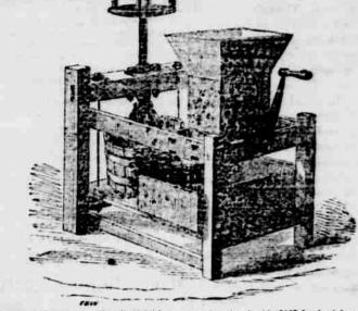
N the present arrangement of this highly approved and valuable MILL, the labor is divided by arranging a cutting Cylinder to beak the apples, and then deliver them to the lower cylinders to be reduced to pomace. By this arrangement the work is performed faster and with much lass
