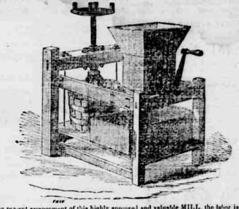
N the present arrangement of this highly approved and valuable MILL, the labor is divided by arranging a cutting Cylinder to break the apples, and then deliver them to the lower cylinders to be reduced to former. By this arrangement the work is performed faster and with much less
