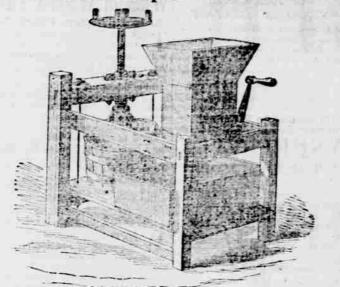
The Cylinders are covered with heavy sheet Zine, both on their peripheries and ends; the wood in them is arranged so as not to swell, and the whole work on the Mill and Press made in the very
