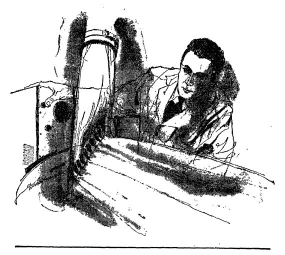
General Motors engineers measure the torque and efficiency characteristics of torque converter blade designs with high velocity fluid flow, using electronic measurement devices to solve for unknowns in highly complex mathematic design problems.
