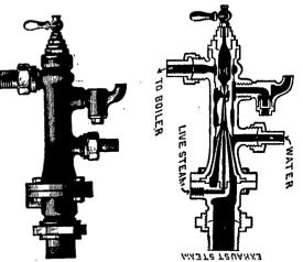
worked by exhaust steam from non-condensing engines.
