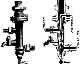
Worked by exhaust steam from non-condensing engines. Is beyond doubt the most economical boller feeder in the market. For particulars address
