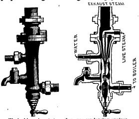
Worked by exhaust steam from non-condensing engines, Is beyond doubt the most economical boiler feeder in the market. For particulars address
