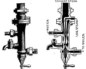
Worked by exhaust steam from non-condensing engines. Is beyond doubt the most economical boller feeder in the market. For particulars address
