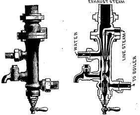
Worked by exhaust steam from non-condensing engines. Is beyond doubt the most economical boiler feeder in the market. For particulars address
