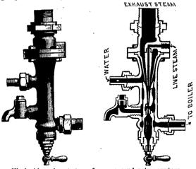
Worked by exhaust steam from non-condensing engines.
