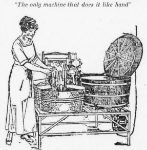
Revolving tub actually RUBS clothing against veighted disc. Process just like hand. Large steel bench accommodates the three tubs and a basket. No stooping or lifting.
