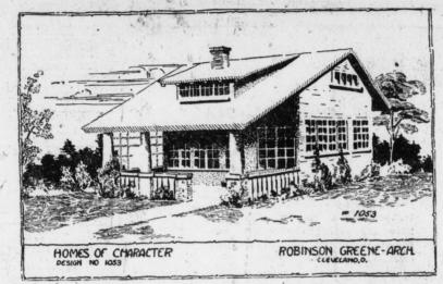
Keeping this time to 26x26 ft., and with a large but secluded porch. The double fireplace between the livingroom and diningroom, which adds to the effect of both rooms while keeping to the cost of but one chimney. There is a built-in buffet, flanked by chimney cabinets, and the bath is accessible from both kitchen and bedroom.
