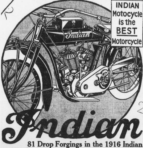
DROP forgings alone—costly to make as they are—meet Indian ideals of strength and stamina where durability and strength are most needed. They are used because they are tougher than castings and more dependable
