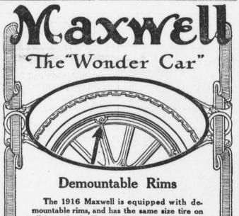
To replace a tire on the road it is only necessary to loosen five bolts; slip off the flat tire; slip on spare rim and tire; tighten three bolts, and proceed.
