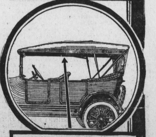
Perfect-fitting, "one-man" mohair top; quick adjustable storm curtains, rolled up inside of top.
