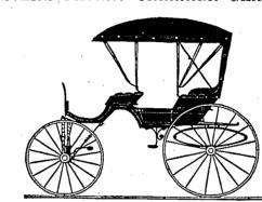
This mode of gearing is far superior to any yet invented for beauty, simplicity and durability, and es not require a genius to attach it to any klad of spring carriage or wagon, and will answer all e purposes that platform gearing will, with about one-fourth the labor.
