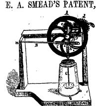
For Converting Rotary into Reciprocating Motion, and Vice Versa.
