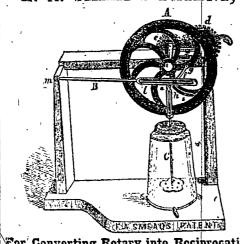
For Converting Retary into Reciprocating Motion, and Vice Versa. PATENTED FEBRUARY 15, 1859
