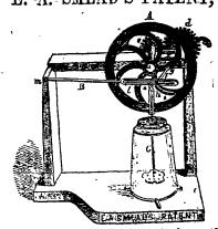
For Converting Rotary into Reciprocating Motion, and Vice Versa. PATENTED FEBRUARY 15, 1859.
