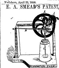
For Converting Rotary into Reciprocating
