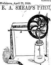
EA SMEAD'S PATENT For Converting Rotary into Recipious Motion, and Vice Versa.
