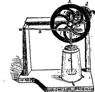
For Converting Rotary into Reciprocating Motion, and Vice Versa. PATENTED FEBRCARY 15, 1859.
