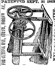
The merits of this machine consists in part, in the attachment of curved knives to the arms of the cutting-wheel, the shearing cut across the mouth-piece, the great power and directness of the blow, by which treble the volume of material is cut, with less power than is required by any other machine; those combined with its durability and simplicity of construction, command public attention. Nothing liable to get our of order, but what a boy could remedy with
