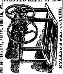
The merits of this machine consists in part, in the attachment of curved knives to the arms of the cutting wheel, the shear-ing cut across the mouth-piece, the great power and directness of the blow, by which treble the volume of material is cut, with machine: those combined with its durability and simplicity of construction, command public attention. Nothing liable to get out of order, but what a boy could remedy with
